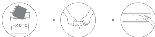
Figure 9 — Cleaning the indoor unit housing
